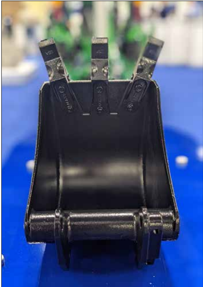
The 2022 Casting of the Year was manufactured by Waupaca Foundry Plants 4 and 5 (Marquette, Wisconsin, and Tell City, Indiana). The first-to-market cast iron bucket attachment for a compact utility tractor replaced a steel fabricated bucket with 159 inches of weldment.
