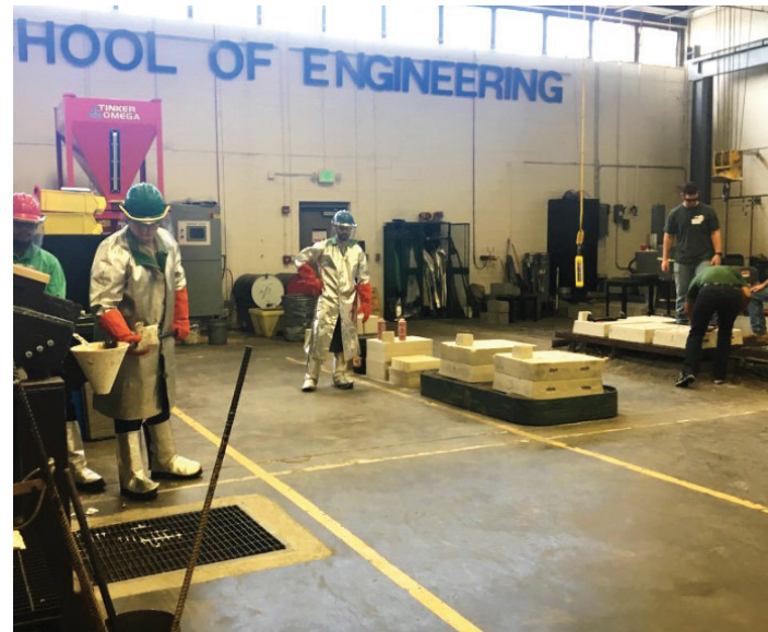
At the seminar, UAB provided a demonstration of 3-D printing tooling and application with both green sand and nobake molds.
