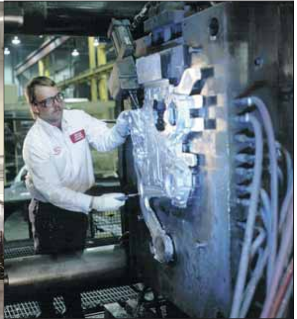
In the diecasting process, metal is ladled into shot sleeves and forced under extreme pressure into the permanent mold or die.
