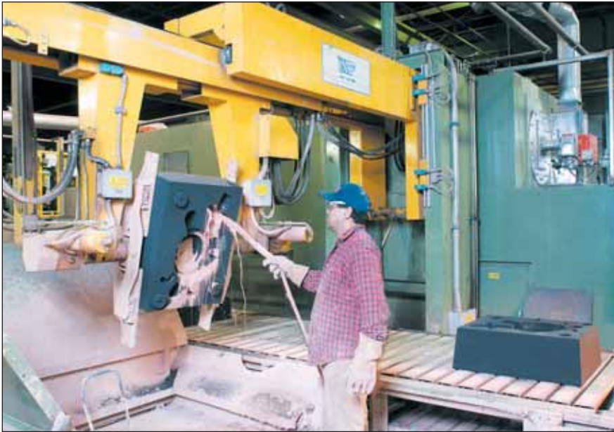
In the nobake molding process, refractory sand is coated with binder and a liquid catalyst. As the binder and catalyst combine, a chemical reaction hardens the sand. Shown above is the application of the refractory coating.
