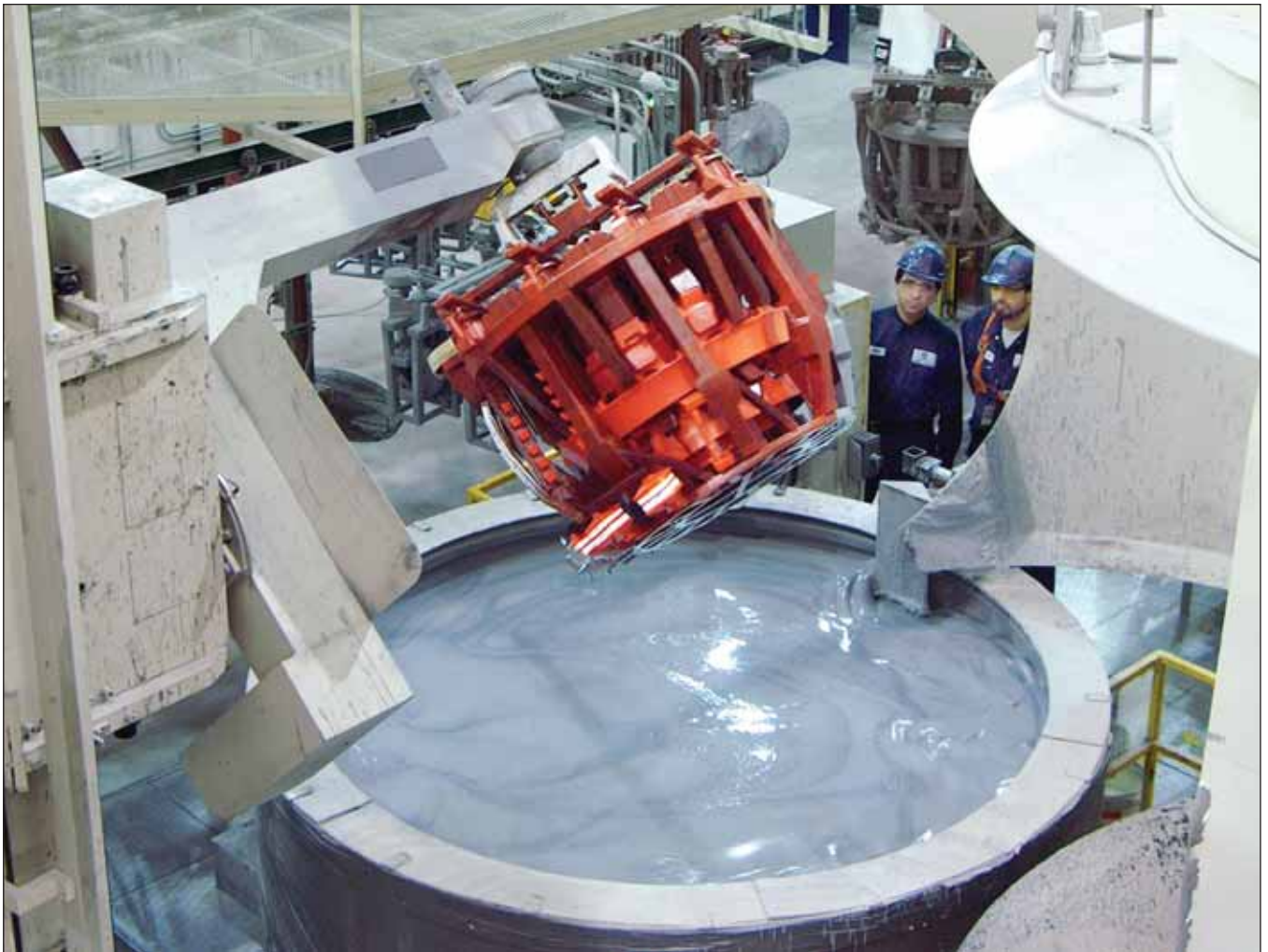
In the investment casting process, wax patterns are produced in dies and assembled. They are then “invested” with ceramic to produce a monolithic mold. The pattern then is melted to leave a precise mold cavity.
