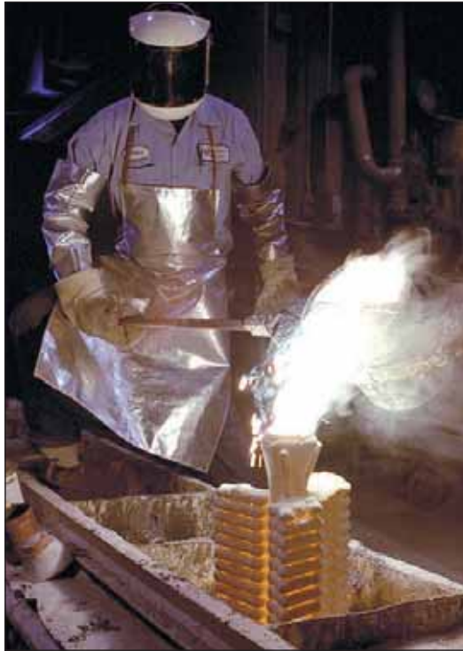
In investment casting, the pattern is covered with ceramic to produce a monolithic mold. When the wax pattern is melted, a precise mold cavity is formed.
