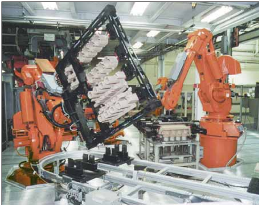
This robot coldbox core and mold making cell is composed of 11 robot arms and gantries designed to automatically produce, assemble and refractory coat components. It requires two operators for inspection purposes.
