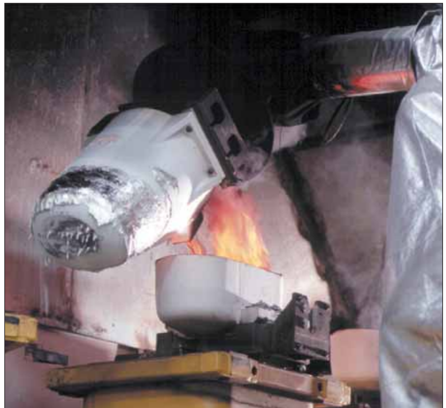
When design engineers are discussing the most efficient molding method to obtain the cast components, they must be familiar with what alloys will be used. Aluminum, shown above during a pouring operation, is a versatile material that can be cast in most types of molds.
