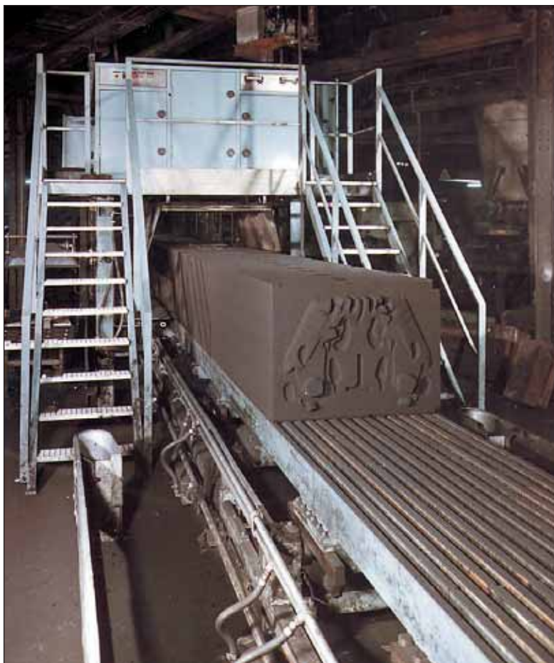
Vertically parted molding machines, normally used for high-production runs, are automated and compact molding sand by squeezing.
