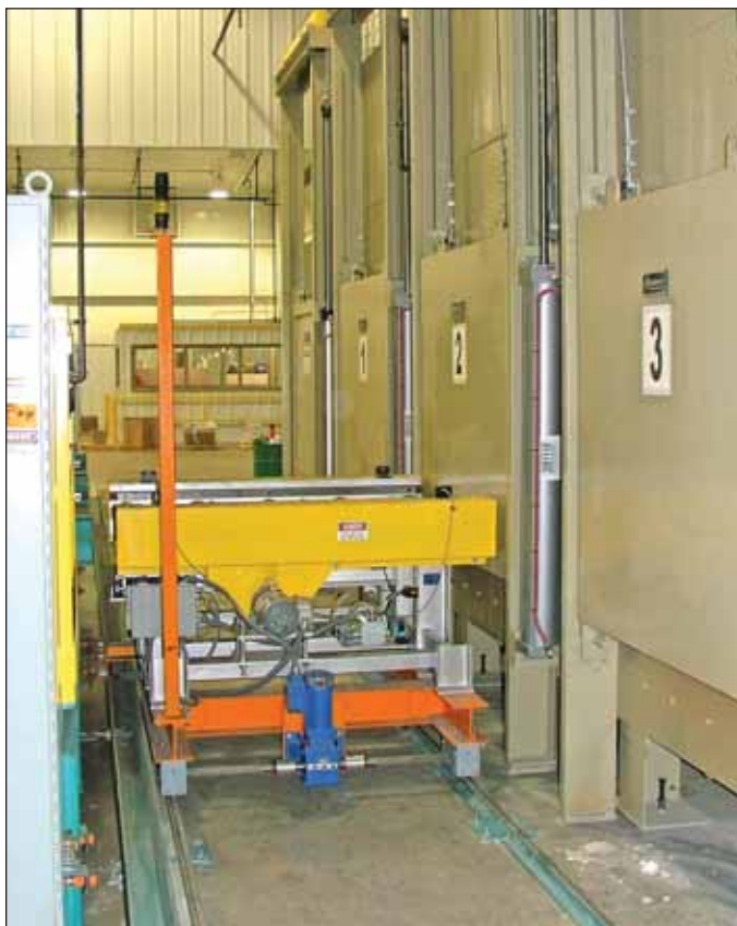
Farrar Corp.'s new annealing station, which includes three furnaces, can handle 2 million lbs. of castings per year and is at 75% capacity.
